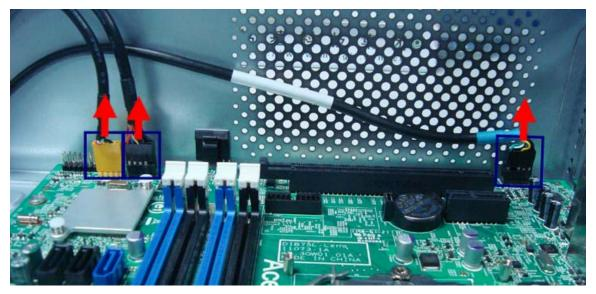
4. Detach the cables from the front I/O and optional card reader. Remove the cables.
